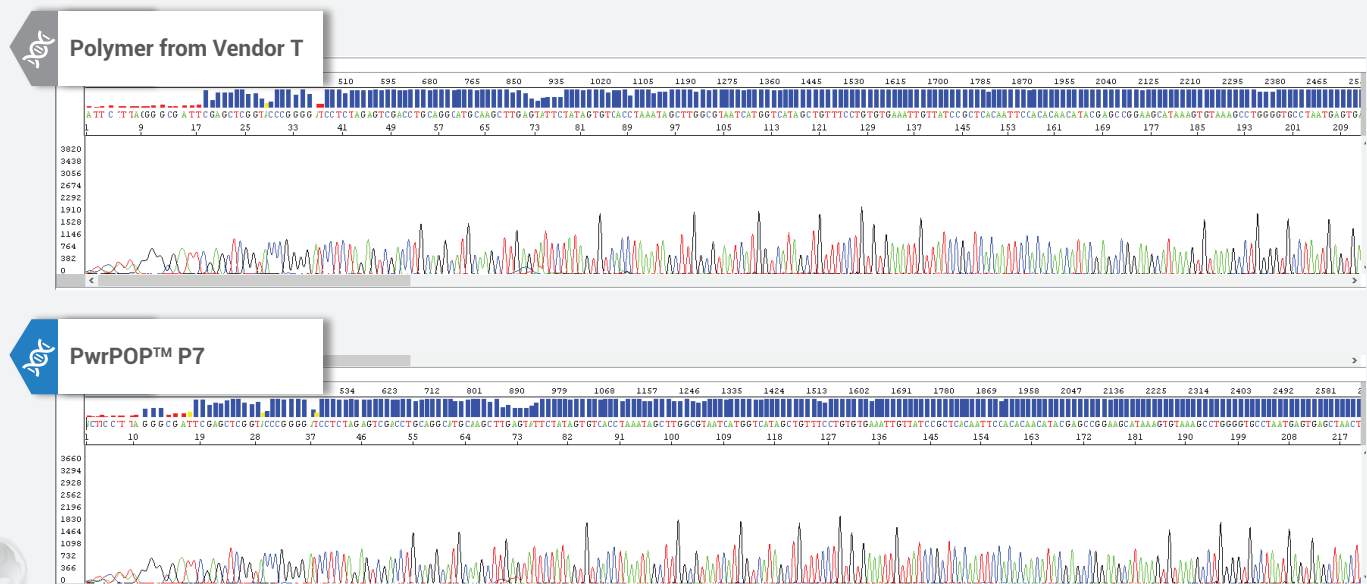
PwrPOP™ P7 Polymer (bottom panel) shows comparative separation performance with Polymer from Vendor T (top panel).
