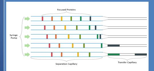
The process of transferring a small section of focused protein into a much longer section effectively minimises the potential remixing of separated proteins inside the transfer capillary. During syringe mobilisation, the electric field can be adjusted to preserve the separation resolution. The difference in capillary ID greatly minimises the remixing of separated protein isomers. Therefore, the resolution achieved during CIEF will essentially be preserved.
