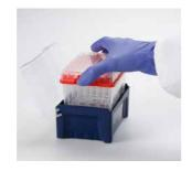
Hold both the refill and the cover by the finger tabs and place inside an empty TipOne® rack until the tabs click into place.
