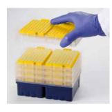
Remove each layer once you have used the tips to reveal the new layer of tips
