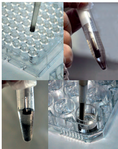
Left: extended magnet and tip without any particles. Middle: particles collected only on the apex of the tip. Right: a larger amount of particles collected using the full power of the magnet.
