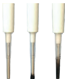
Left: extended magnet and tip without any particles. Middle: particles collected only on the apex of the tip. Right: a larger amount of particles collected using the full power of the magnet.
