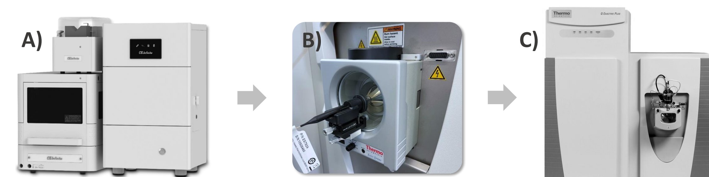
Fig 3. A) The transfer capillary from CEInfinite is coupled to the B) Thermo EASY-Spray Ion Source coupling using a nanospray adapter developed by AES. C) This interface connects directly to the Thermo Q Exactive Plus mass spectrometer with the entire setup taking approximately 5 min to complete.
